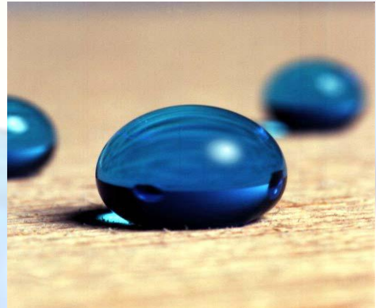
Water droplets on a wood surface treated with BASF's "Lotus Spray". Image Courtesy of BASF, Germany.
